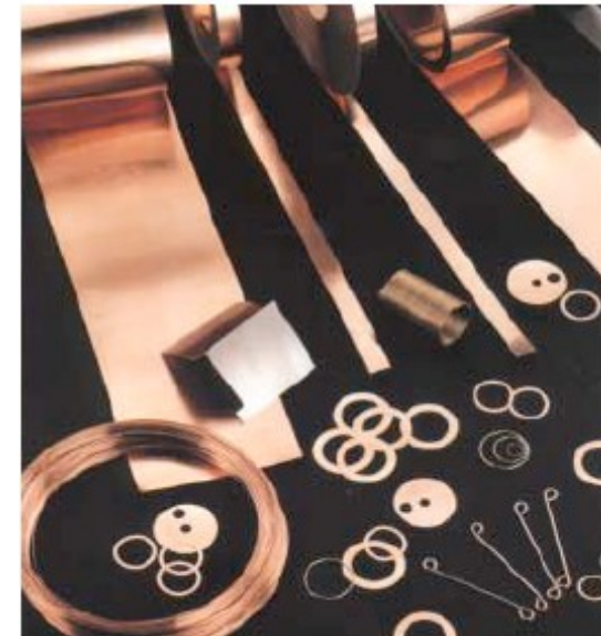
Figure 11. Typical brazing filler metal preforms. (Photo courtesy of Handy & Harman)
