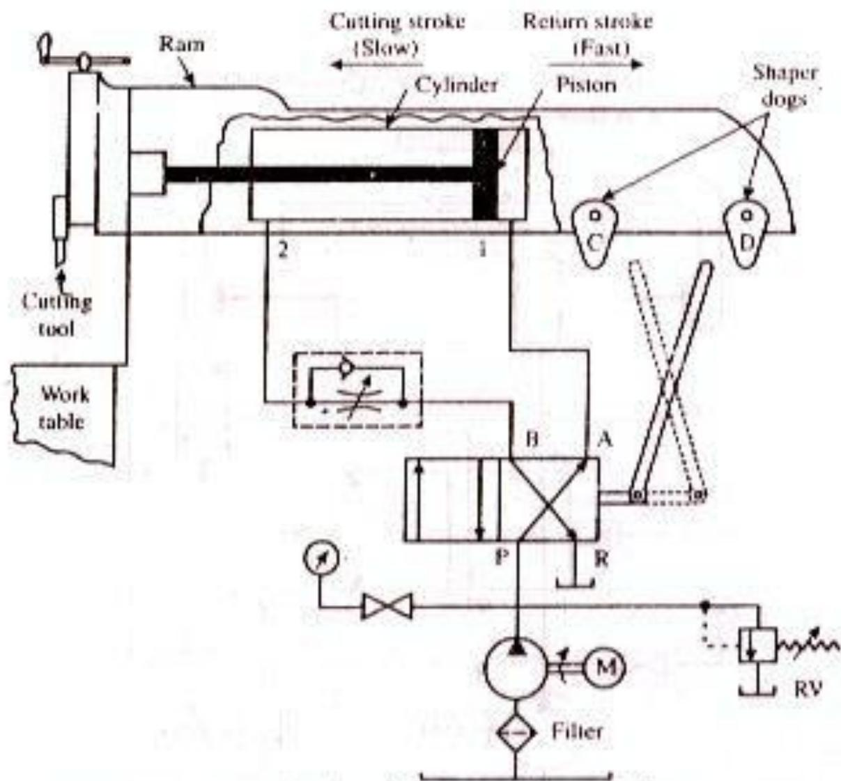
**Fig. 7.14 : Hydraulic circuit for operation of shaper**
