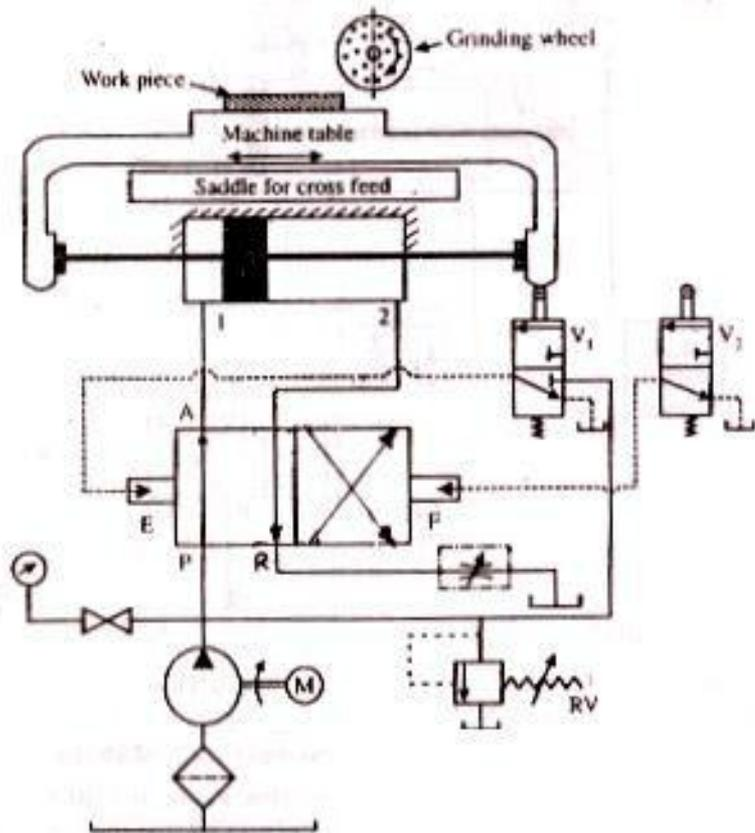
Fig. 7.15 : Hydraulic circuit for surface grinder
