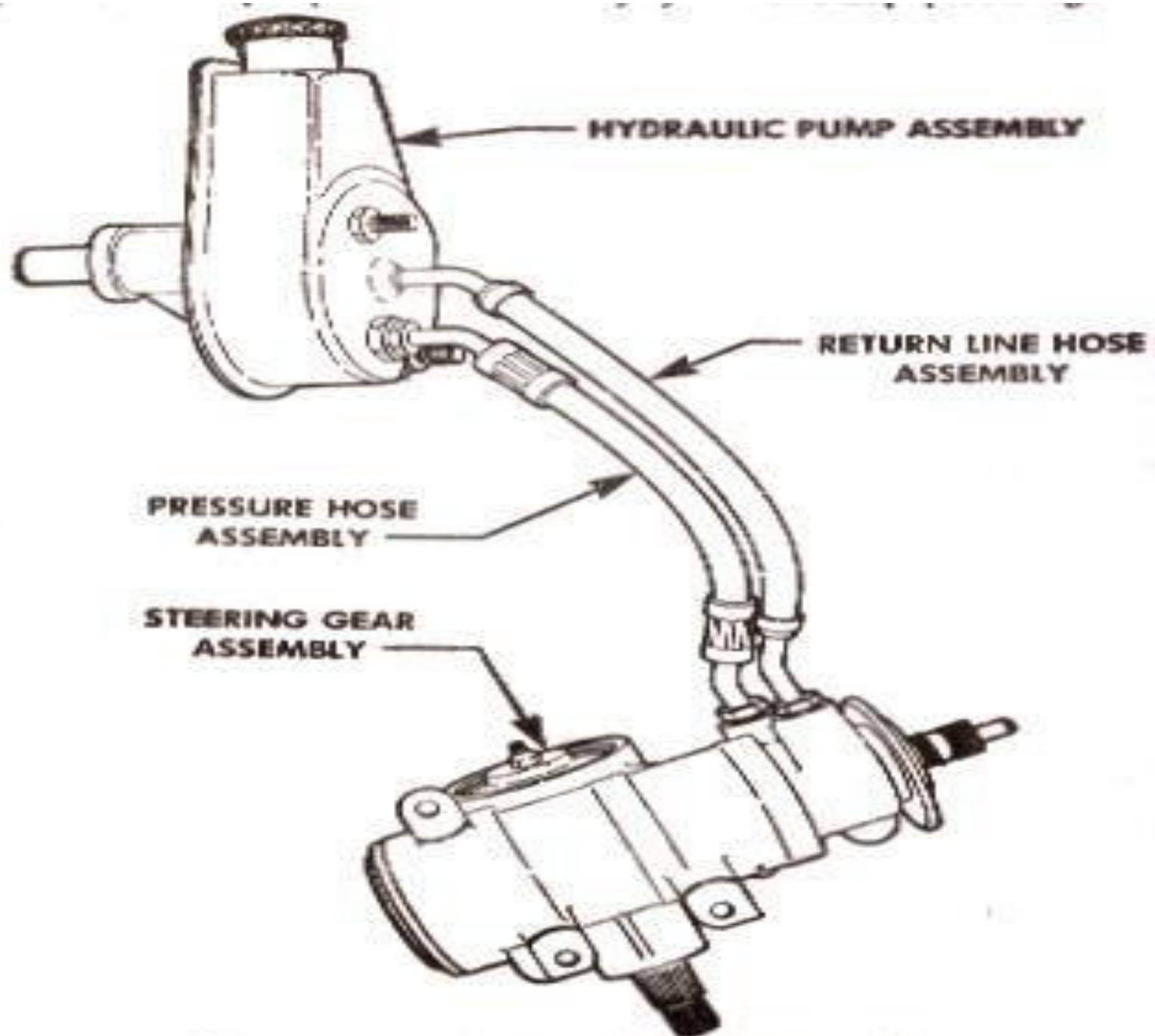
Fig. 8.56. Layout of an integral power steering system.
