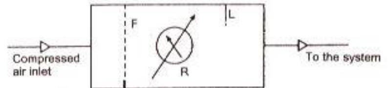
**Fig. 12.2 : Simplified pneumatic power unit**
