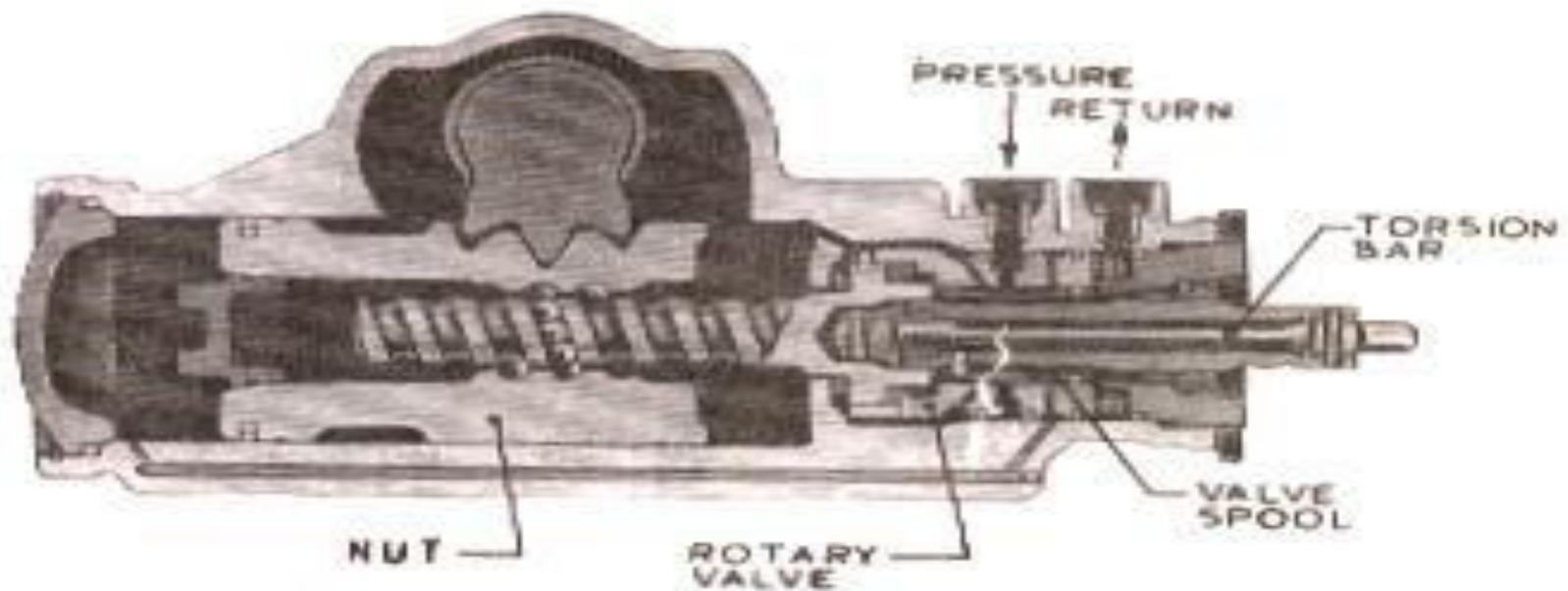
Fig. 8.57. Rotary valve power steering gear
