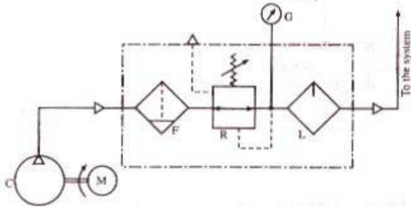
G - Pressure gauge, R - Regulator, F - Filter, M - Electric motor,
