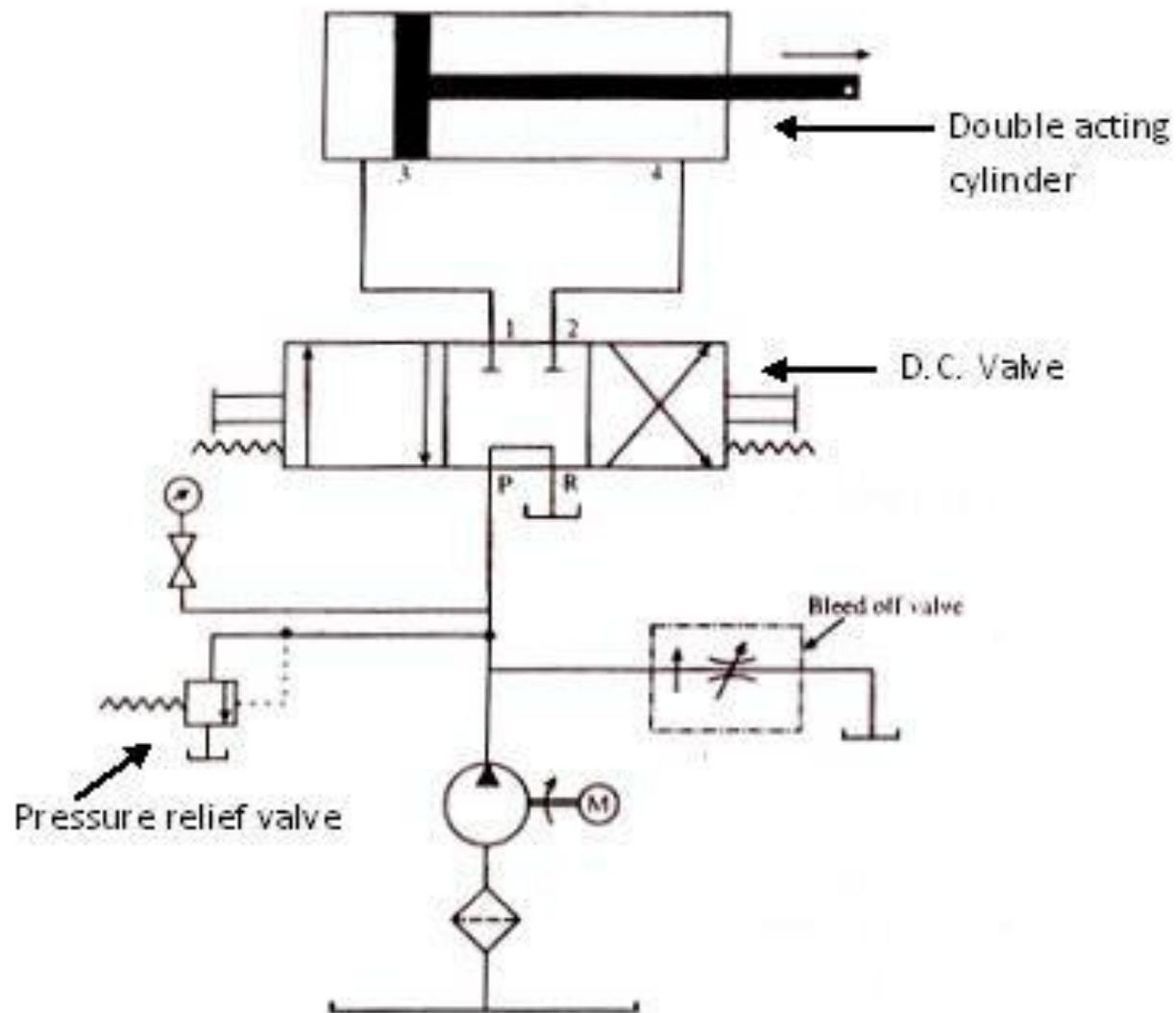
**Fig. 7.6 : Bleed-off speed control hydraulic circuit**
