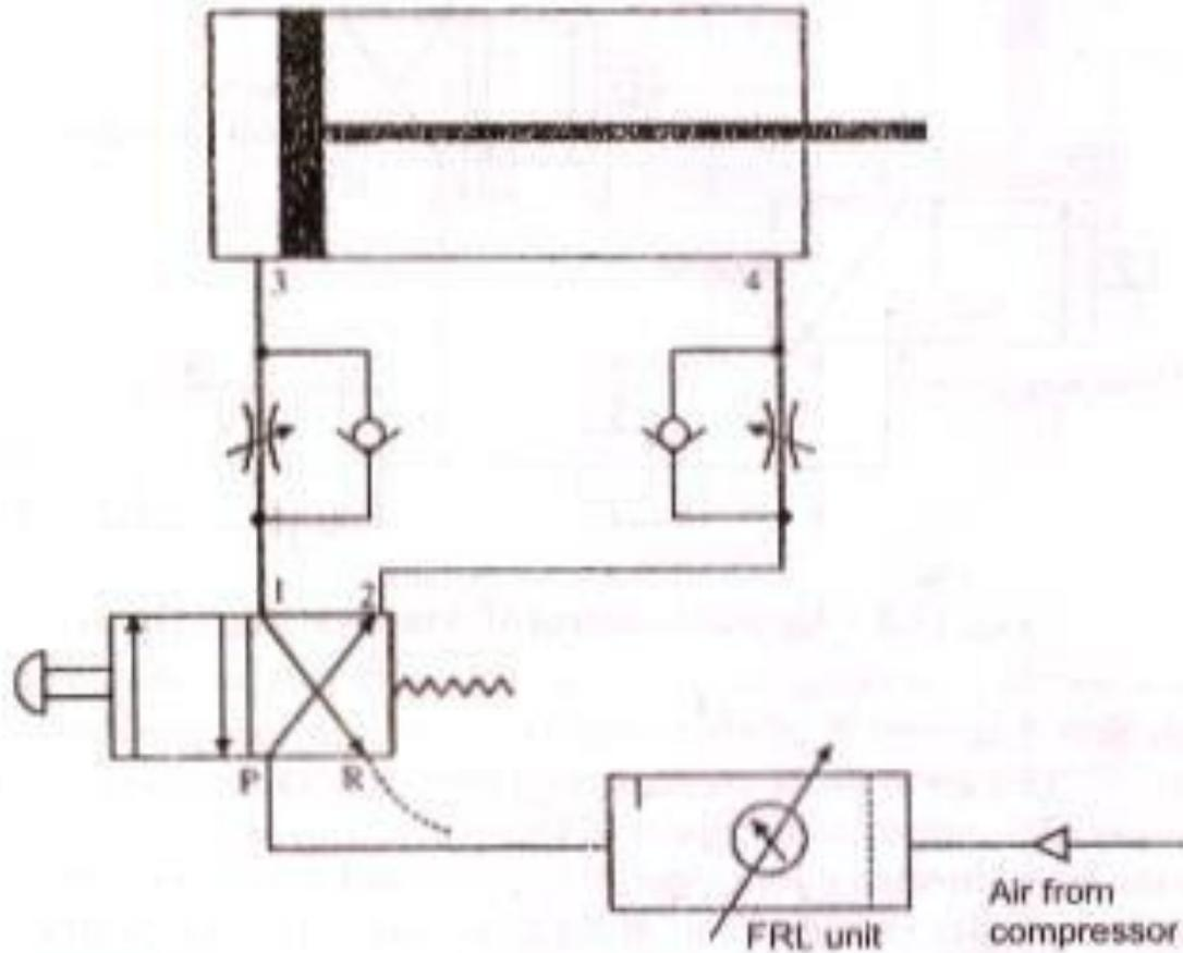
**12.7 : Pneumatic circuit of control speed of double acting cylinder**
