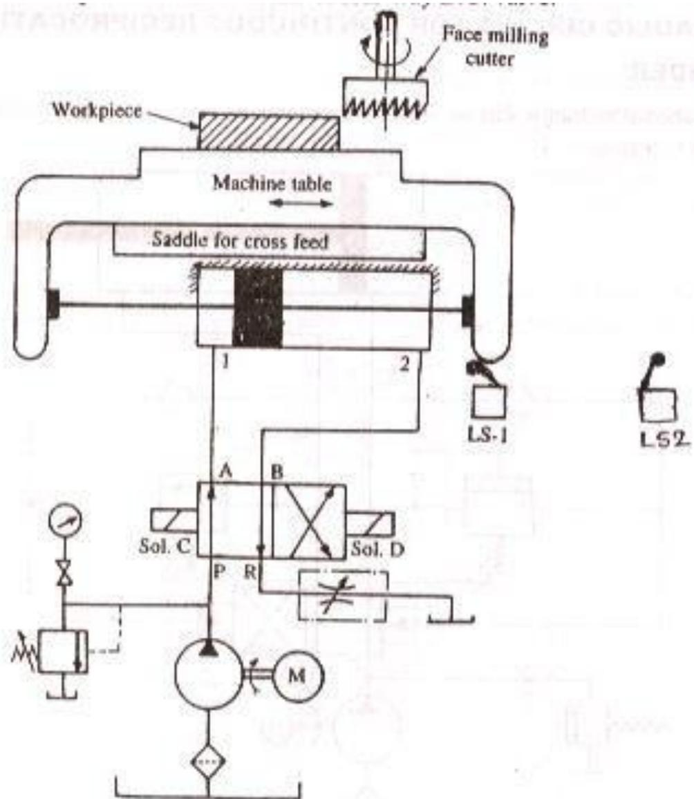
Fig. 7.13 : Hydraulic circuit for milling machine
