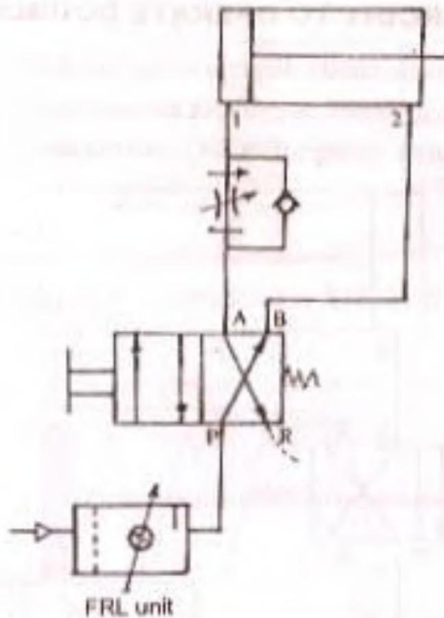
**Fig. 12.5 : Pneumatic circuit used for meter-in applications**
