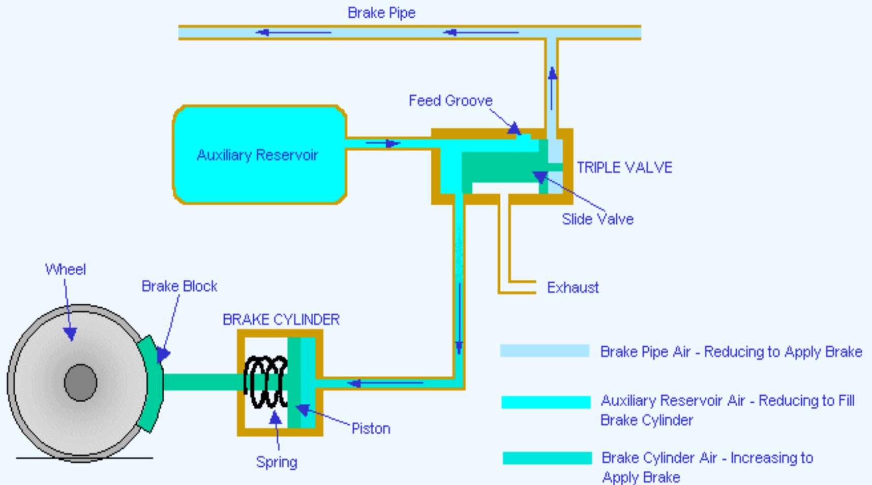
**Schematic Diagram of Air Brake System on Vehicle in Application Position**
