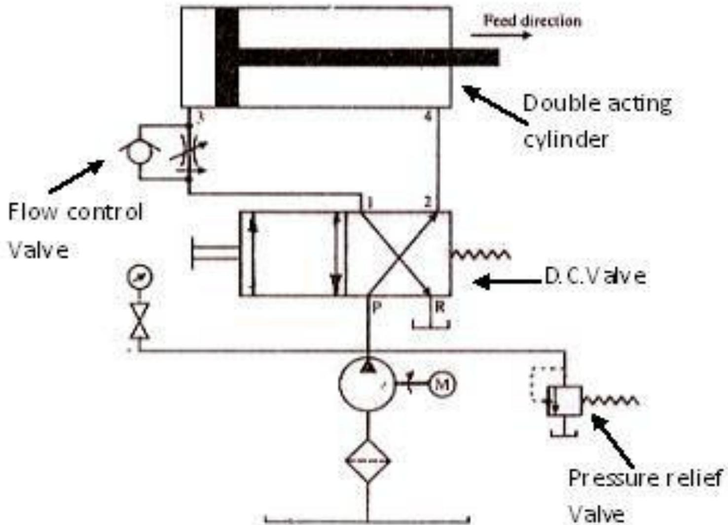
Fig. 7.3 : Meter-in hydraulic circuit
