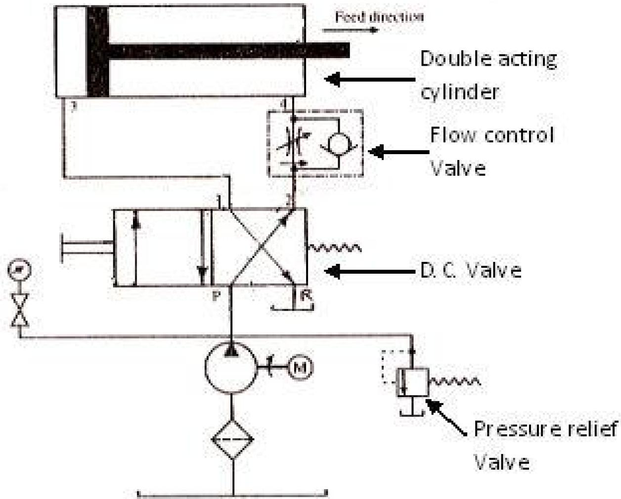
**Fig. 7.4 : Meter-out speed control hydraulic circuit**
