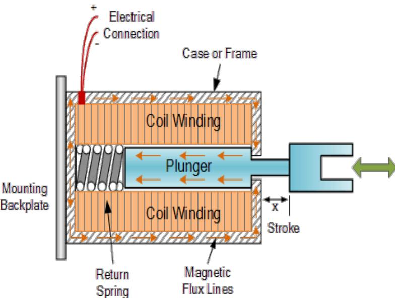
A **solenoid valve** is an electromechanically operated valve. The valve is controlled by an electric current through a solenoid: in the case of a two-port valve the flow is switched on or off; in the case of a three-port valve, the outflow is switched between the two outlet ports. Multiple solenoid valves can be placed together on a manifold.
