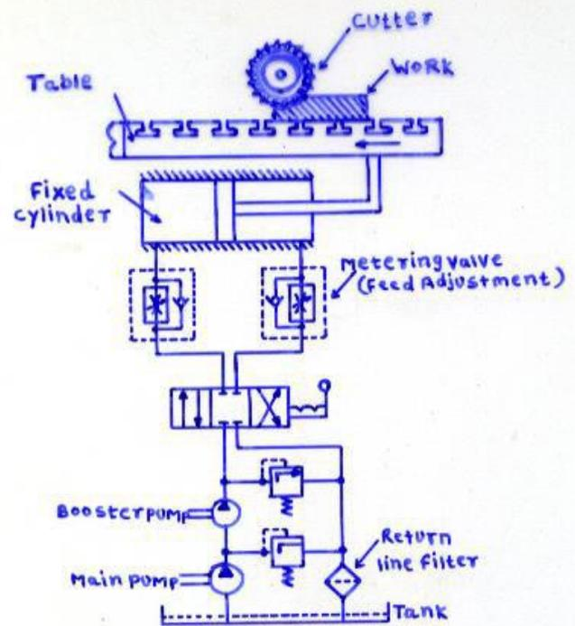
Hydraulic circuit for milling machines.
