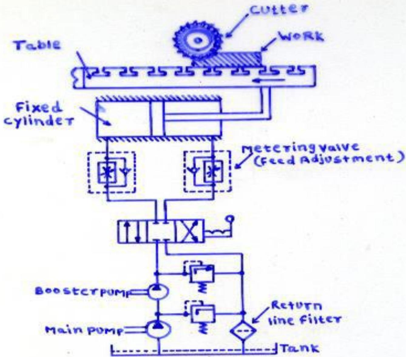
Hydraulic circuit for Milling machines.
