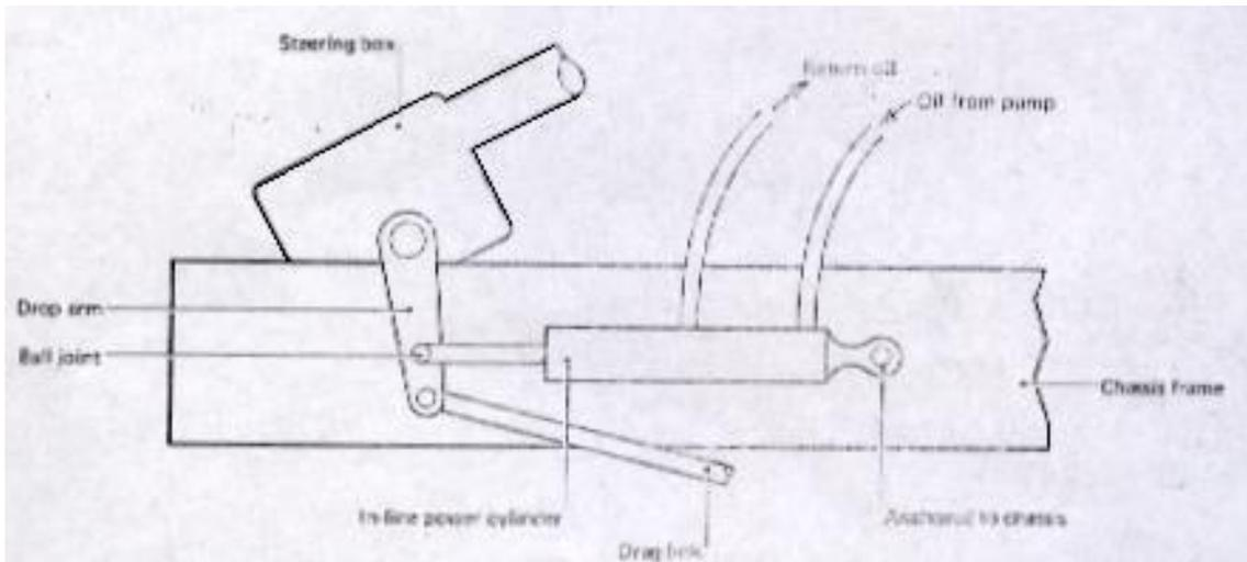
Figure 278(a) Connection of in-line booster.
