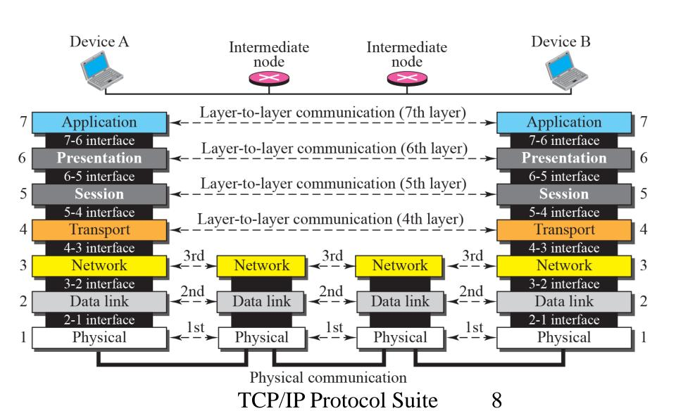
Figure 2.5 An exchange using the OSI model
