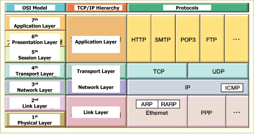
Link Layer : includes device driver and network interface card
